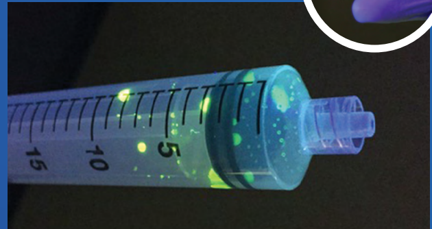
Syringe contamination can be demonstrated using fluorescein and a gloved hand. With repeated emptying and refilling of the syringe, fluorescein travels past the plunger.
